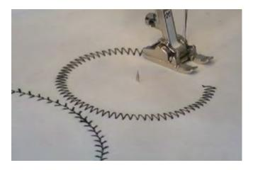
By sliding the pin to a different position, you can change the size of the circle.
