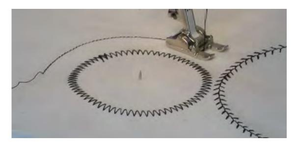
If you leave the fabric on the pin and just change the location of the pin, you create concentric circles because you are using the same pivot point.
