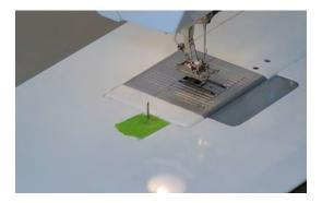
Tape the tack (point up) to the bed of the machine. Use painter's tape because it doesn't leave sticky residue behind.
