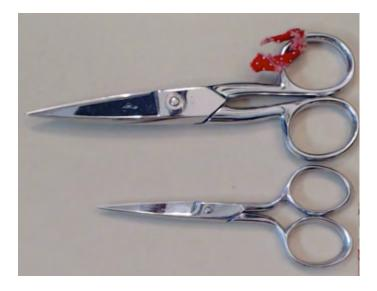
The top scissor is the 5" Gingher. The bottom is the **3" trimming scissor** by Gingher. You can see a big difference in the thickness of the cutting blades as well as a difference in the handle loop size. You need both if you sew very much. The small one is good for clipping threads around your sewing machine. Both of these scissors come with protective sheaths. Keep them covered when not in use to protect the tips.
