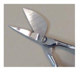
**Appliqué (or duck-bill) scissors** are a must have if you do machine appliqué. The bigger blade helps protect the base fabric when you trim away the top fabric.
