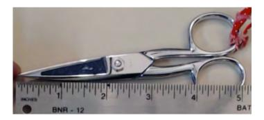
This **5" scissor** is also made by Gingher. It's very sharp and great for clipping, trimming and grading seams.
